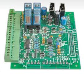
EL-Actuator: IT 100 R Voltage, U 24 Vdc Current, Imax 6 AMP
